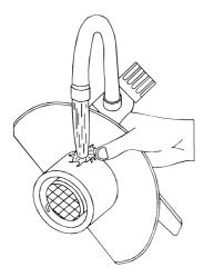
**Removal & Cleaning -** Unlock the circular filter assembly from the bottom of the tank by rotating counter-clockwise and lifting on its handle. No further disassembly is necessary.
